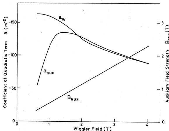
Fig. 1 Coefficient of the quadratic term of the radial distribution of the UVSOR wiggler depends on the field strength.  $a_w$  is the value at the peak of the main field and  $a_{aux}$  is that of the auxiliary field. The auxiliary field strength  $B_{aux}$  is nearly proportional to the strength of the wiggler field.
