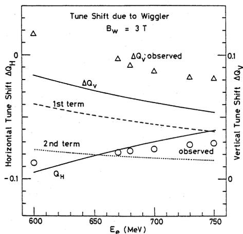
Fig. 5 Tune shifts depend on the beam energy. In this case the field strength of the wiggler is 3 T. Broken and dotted lines are the first and second terms of Eq. (2).
