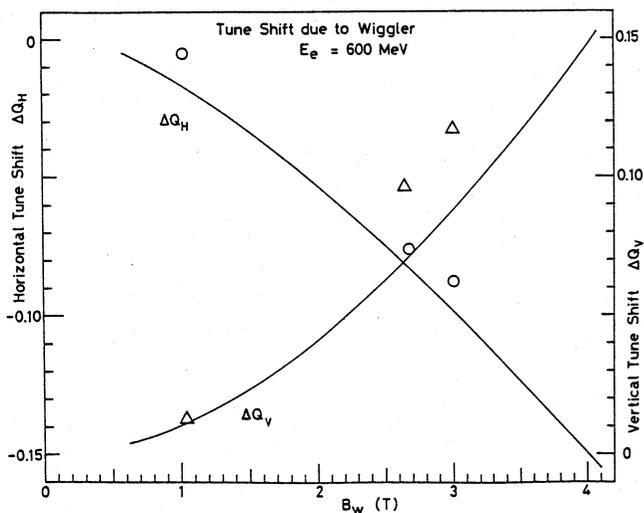
Fig. 3 Tune shifts due to the wiggler depend on the field strength. The beam energy is 600 MeV.
