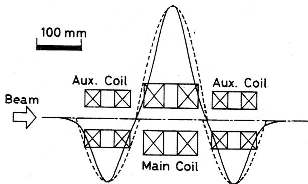
Fig. 2 Vertical field of the UVSOR wiggler along the longitudinal direction.
