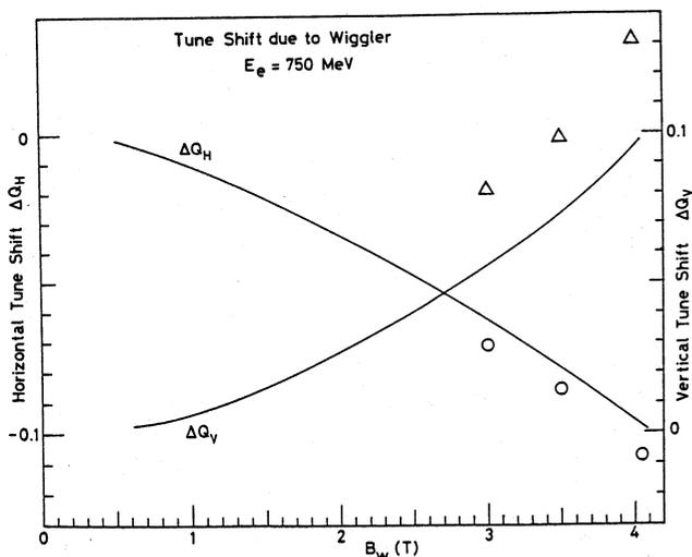
Fig. 4 Tune shifts due to the wiggler depend on the field strength. The beam energy is 750 MeV.
