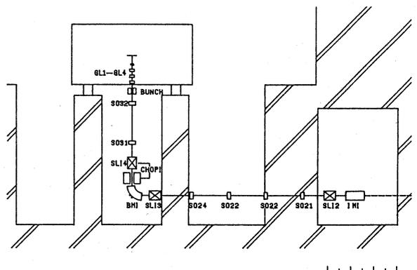
Fig. 2 Side View of the Injection System.
