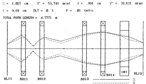
Fig. 4 Beam Envelopes for the Transport Section of the ECR Ion Source.
