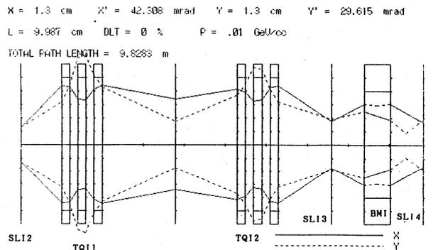
Fig. 6 Beam Envelopes for the Horizontal Transport Section Using two Triplet Quadrupole Magnet Lenses.
