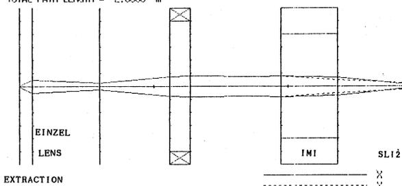
Fig. 9 Beam Envelopes for the Duoplasmatron Ion Source Injection System.
