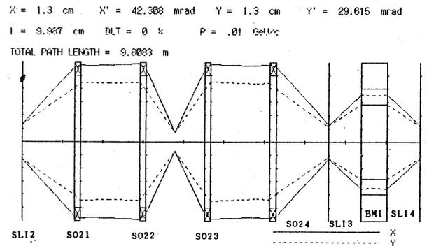
Fig. 5 Beam Envelopes for the Horizontal Transport Section Using four Solenoid Lenses.
