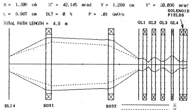
Fig. 7 Beam Envelopes for the Axial Injection Section in the Case of Using four Solenoid Lenses in the Horizontal Transport Section.
