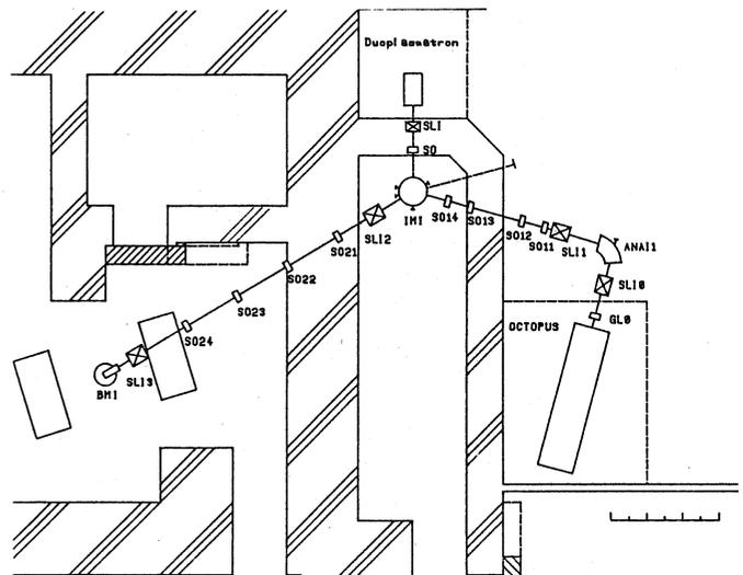
Fig. 1 Top View of the Injection System.
