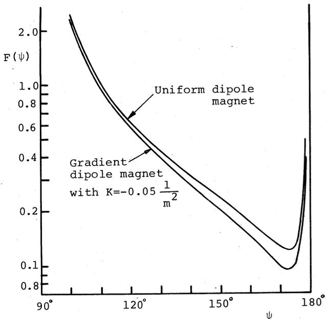
Fig. 2. Form factor  $F(\psi)$  as a function of betatron phase advance per half cell  $\psi$ .
