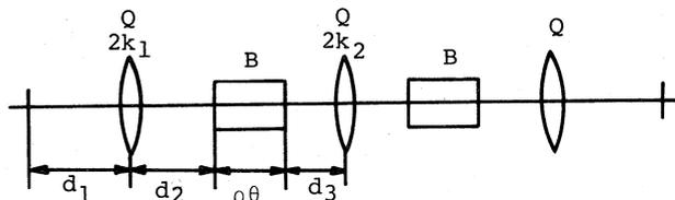
Fig. 1 Schematic Chasman-Green lattice
