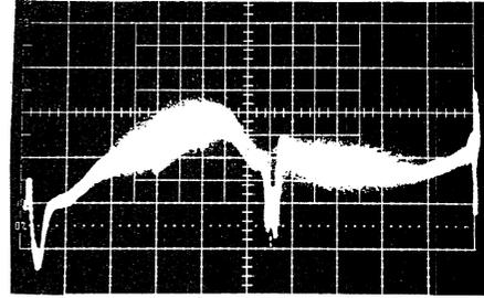
Fig. 5 Signal of MCP at nearest position (Noise and Real signal) 5ms/div, 500mV/div
