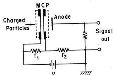
Fig. 2 Electric Circuit to get signal from MCP
