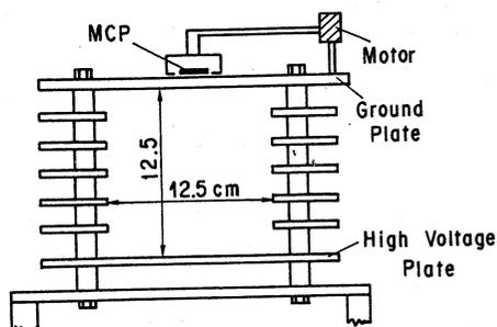
Fig. 1 Schematic of Nondestructive Profile Monitor
