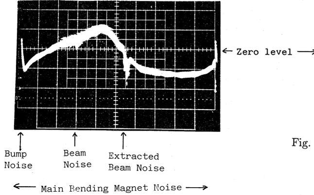
Fig. 4 Signal of MCP at farthest position (Noise)
