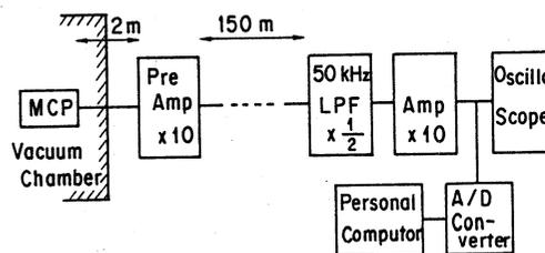
Fig. 3 Electronics System of Nondestructive Profile Monitor
