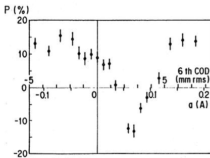
Fig. 7 Harmonic Correction of  $\gamma G = 6$  Resonance.
