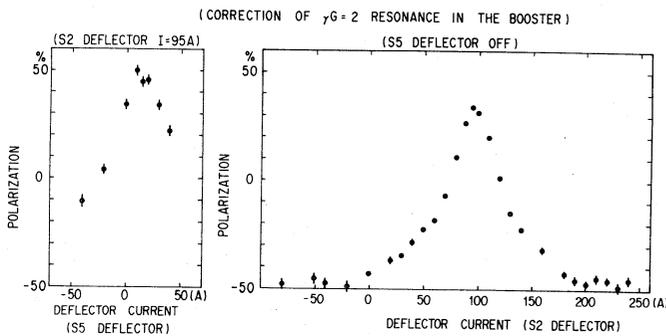
Fig. 3 Harmonic Correction of  $\gamma G = 2$  Resonance.
