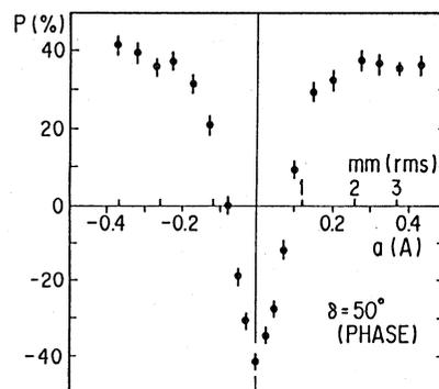
Fig. 9 Harmonic Correction of  $\gamma G = 7$  Resonance.
