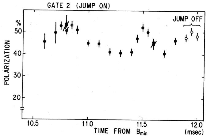
Fig. 4 Tune Jump Correction of  $\gamma G = \nu_x$  Resonance.
