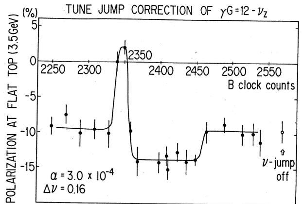
Fig. 5 Tune Jump Correction of  $\gamma G = 12 - \nu_z$  Resonance.
