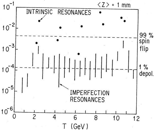
Fig. 2 Resonance Strength in the Main Ring.
