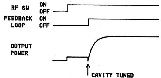
Fig. 5 Start sequence of the voltage control system
