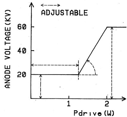
Fig. 4 Anode voltage versus drive power
