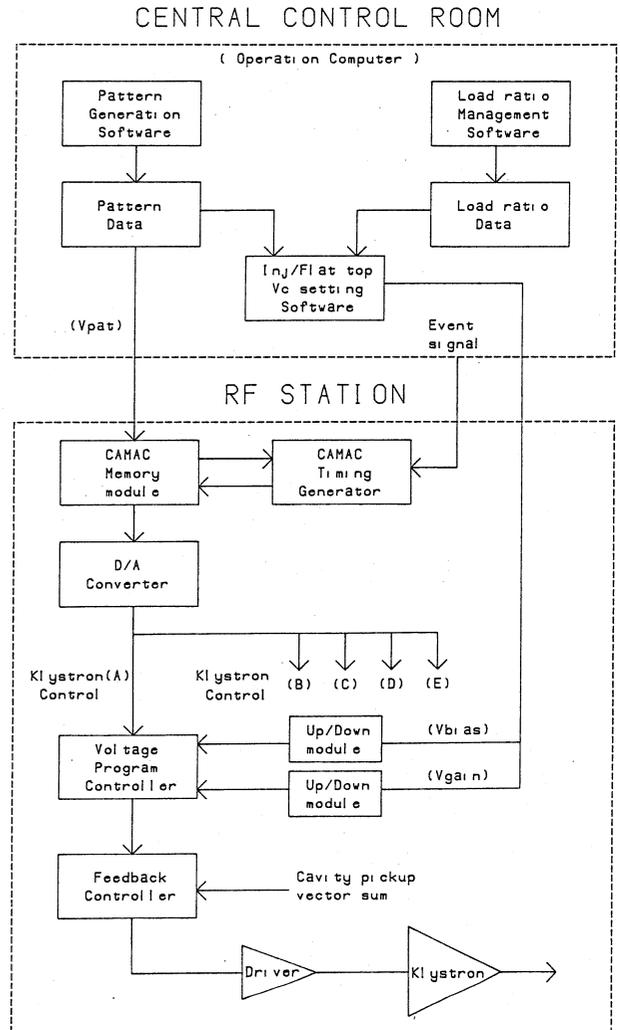
Fig.1 The RF control system for management of the accelerating voltage pattern
