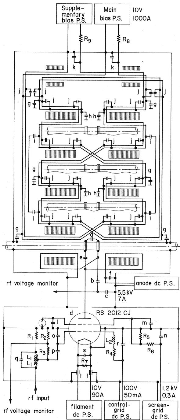
Fig. 1 Schematic electrical configuration of the rf cavity and the final rf power amplifier.
