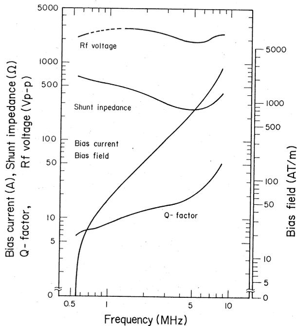
Fig. 2 Rf characteristics of the fundamental resonance of the cavity together with a relation between the ferrite-bias current and the frequency. Q-factor and shunt impedance are reduced from low-level rf measurement. Rf voltage is a peak-to-peak value measured at the right half cavity in preliminary rf power test: a dotted line implies that no clear data has been obtained so far.
