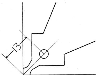
Fig.6 Bead position for bead perturbation method
