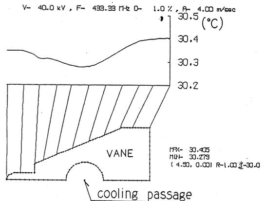
Fig.5 The temperature distribution on RFQ vane cooled by single cooling passage of 20-mm diameter
