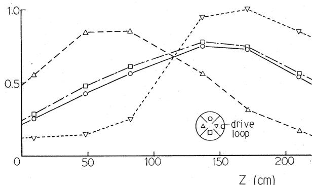
Fig.7 Field distribution in the cavity before adjustment
