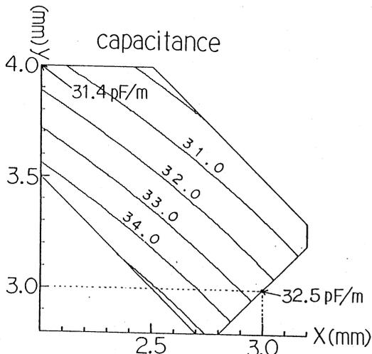
Fig.3 The capacitance contour as a function of  $x$  and  $y$
