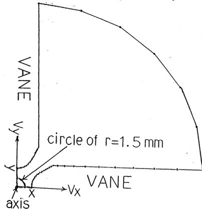
$x, y$ : distance between axis and vanetip
