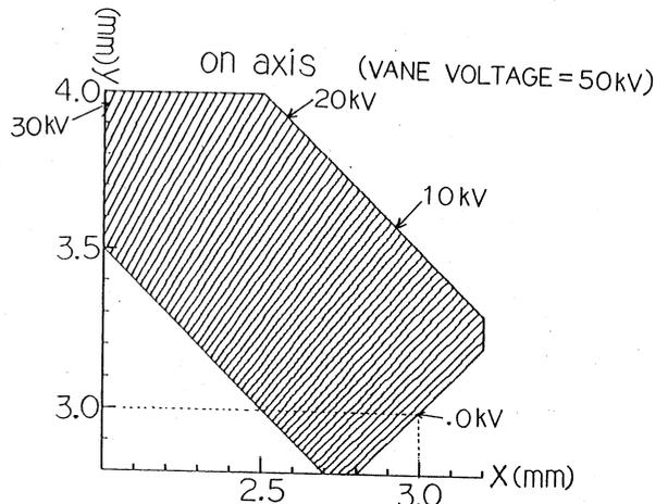
Fig.4 The potential contour on axis
