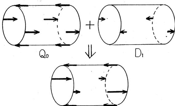
Fig.8 Mode mixing of  $Q_0$  and  $D_1$  mode.
