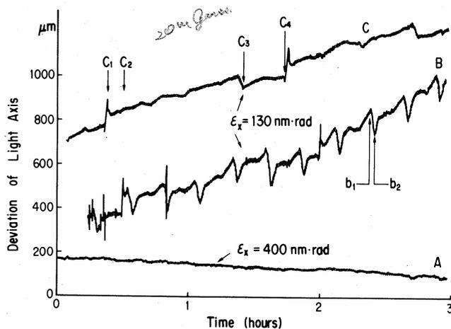
Fig. 3 Vertical deviation of light axis in long term.
