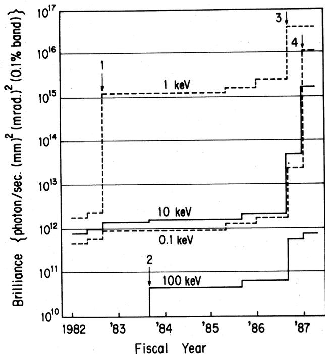
Fig. 5 Available brilliance of SR at the energy from 0.1 KeV to 100 KeV. Numbers indicated in the figure mean ; 1. an undulator was inserted at BL-2, 2. a vertical superconducting wiggler operated. 3. low emittance mode operation started. 4. a multipole wiggler was allocated.
