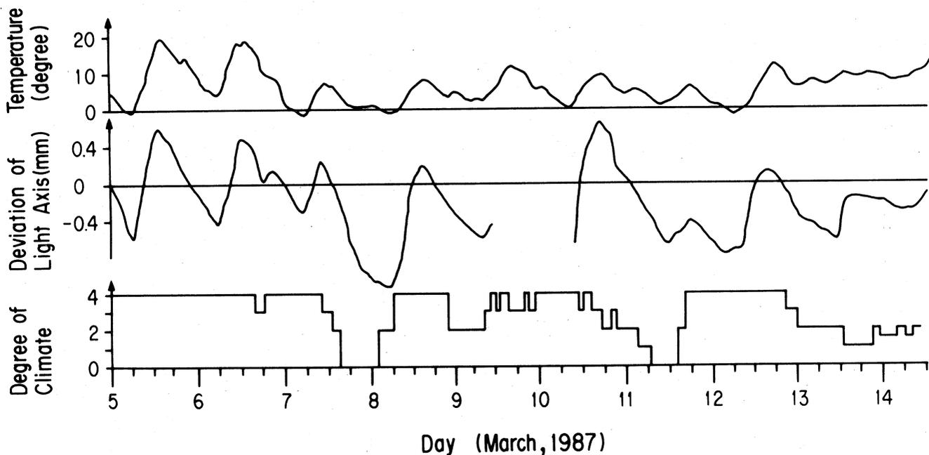
Fig. 4 Correlation between the deviation of the light axis (No.21 channel) and the outdoor temperature and the change of the climate. The deviation was measured at the point 12 m apart from the light source. Degree of climate means : 0 = snowfall, 1 = rainfall, 2 = thick cloud, 4 = thin cloud, 5 = sunshine.
