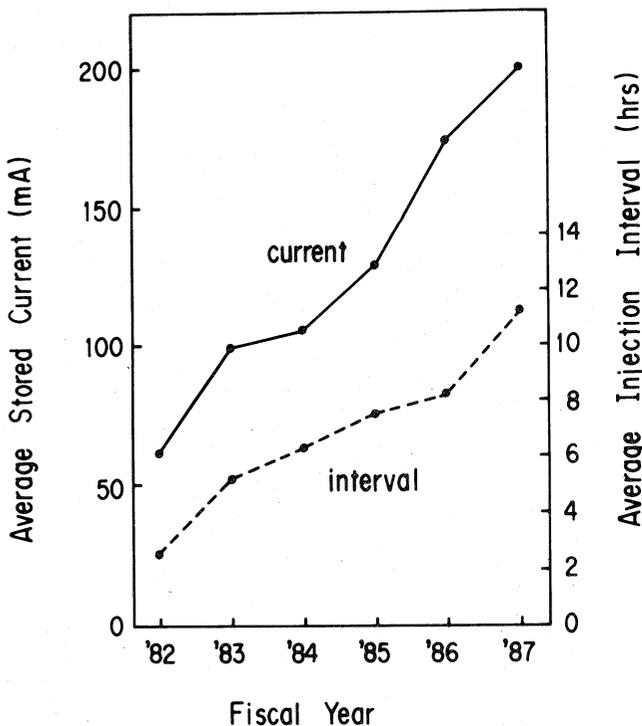
Fig. 2 The average stored current and the average injection interval during user time.
