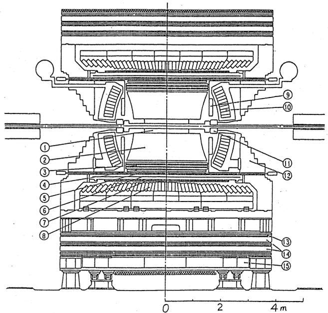
Fig. 2 VENUS detector. (1) and (2) are tracking chambers inside the solenoid (6). They are covered by calorimeters (8) and (10), and by muon detector system (13) and (14).
