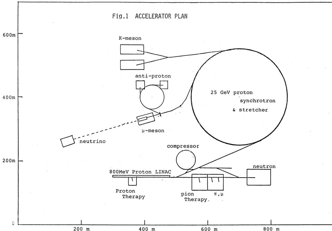
consideration: a combined-type synchrotron may be interesting from the view point of compactness. There may also be substantial advantage for the rf system if a booster accelerator is adopted between the 800 MeV linac and the 25 GeV cynchrotron. Extensive studies of such alternative disigns are now under way, in addition to the feasibility study of the proposed rf system.
