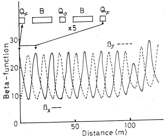
Fig. 3 Beta function and the lattice structure of a normal bending cell
