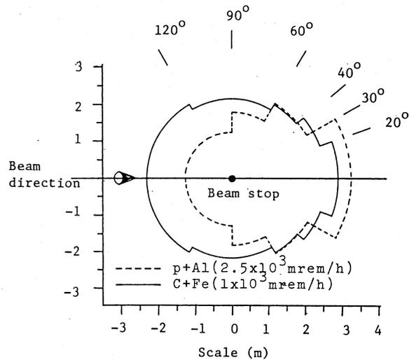
Fig. 4. Iso-dose contours for the sources of p+Al and C+Fe.
