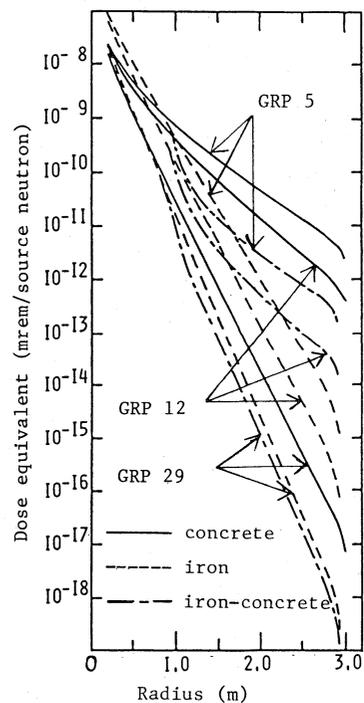
Fig. 2. Dose attenuations in spherical beam dumps.
