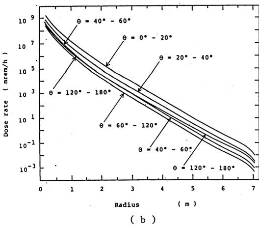
Fig. 3. Dose rates as a function of radius for neutron sources generated by reactions of a) the p+Al and b) the C+Fe. Beam intensity is  $6 \times 10^{12}$  ions/sec. In (a) only the calculated results in angular interval  $0^\circ - 30^\circ$  are given.
