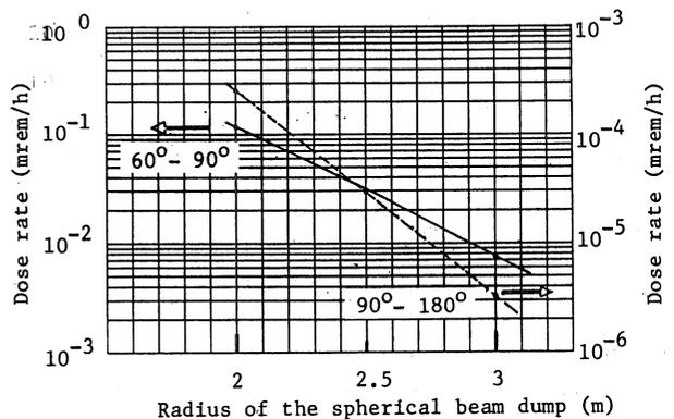
Fig. 5. Dose rate at the outer surface of a concrete spherical shell as a function of the radius of a concrete beam dump for the p+Al. Beam intensity is assumed to be  $6 \times 10^{12}$  ions/h.
