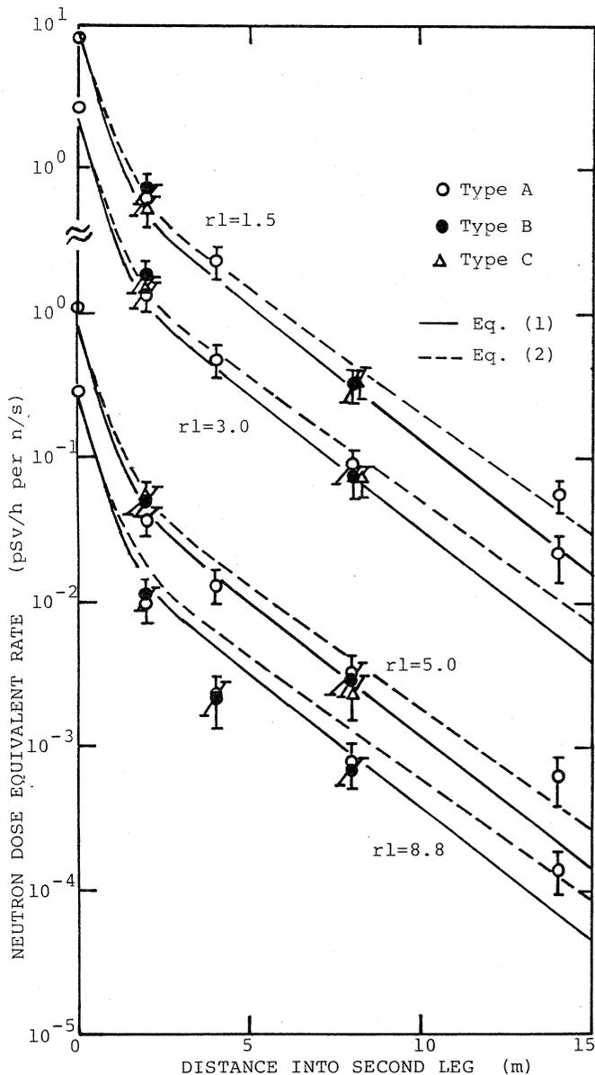
Fig. 3 Attenuation of neutron dose equivalent in the 2nd leg. Length of the each 1st leg is 1.5, 3.0, 5.0 and 8.8 m.
