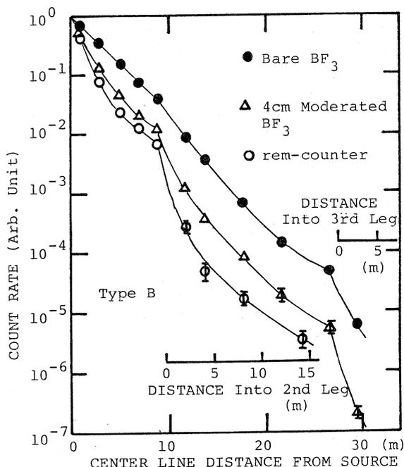
Fig. 1 Attenuation of neutrons in three-legged labyrinth measured by rem-counter, bare BF<sub>3</sub> and 4 cm thick polyethylene moderated BF<sub>3</sub> counters.
