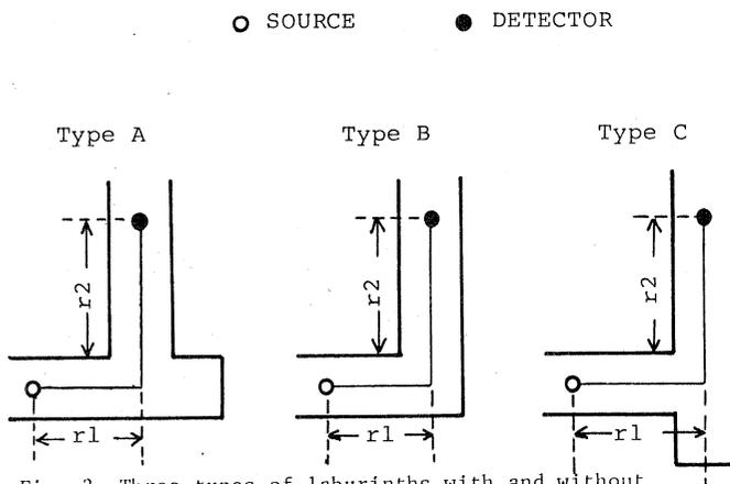
Fig. 2 Three types of labyrinths with and without "neutron traps" at the entrance of the 2nd leg
