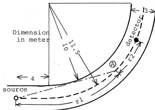
Fig. 4 Curved maze. The source disappears at A.
