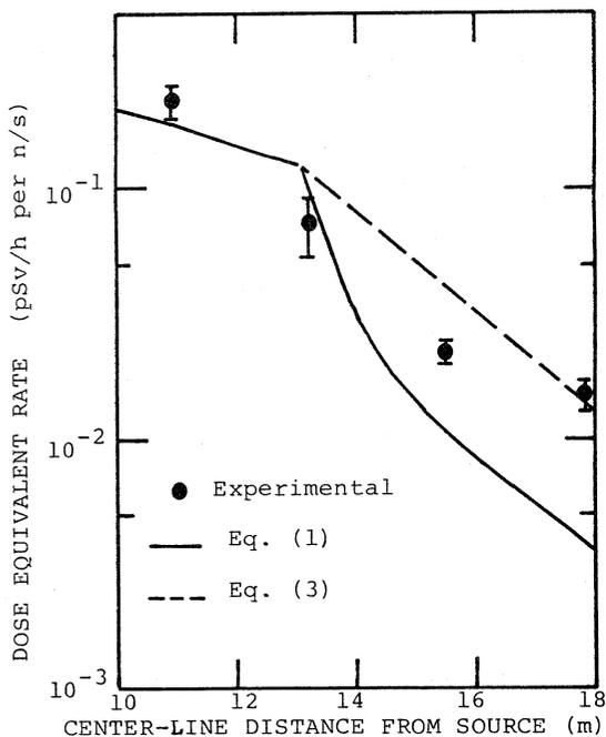
Fig. 5 Dose equivalent rate in curved maze.
