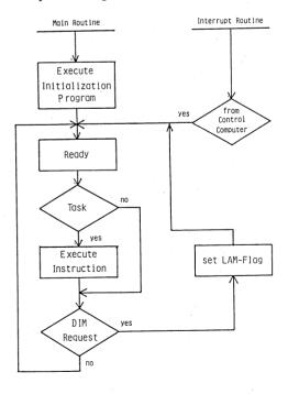
Fig. 1 Operation flow diagram of CIM.
