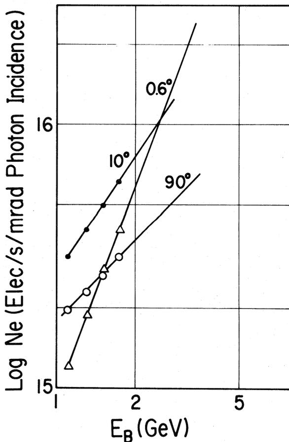
Fig. 4 The beam energy dependence of photoelectrons for 90°, 10° and 0.6° angle of incidence.
