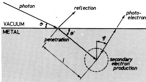
Fig. 1 The schematic drawing of photoelectron production.
