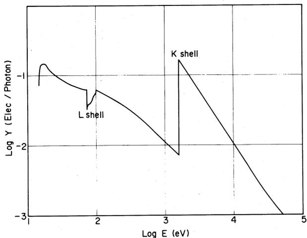
Fig. 2 The photoelectron yield at normal incidence for aluminum.
