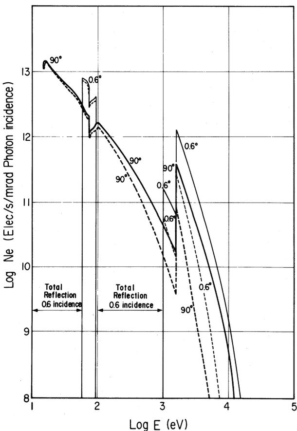
Fig. 3 The number of photoelectrons produced at 1 mrad photon angle of incidence.
