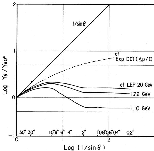
Fig. 5 The angle of incidence dependence of the photoelectron yield. The dashed line shows experimental outgassing rate.
