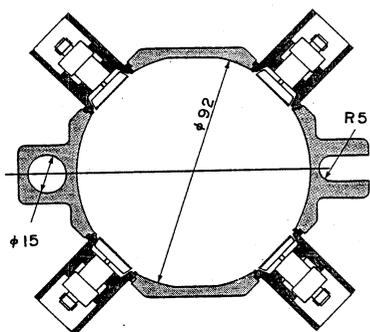
Fig. 3 Straight section chamber with beam position monitor electrodes.
