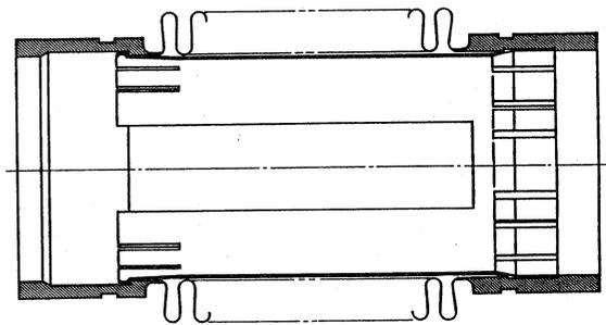
Fig. 2 Racetrack type, aluminum alloy(3004) seamless bellows with rf insert(Be-Cu).
