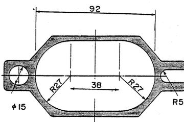
Fig. 4 Straight section chamber for septum magnet.
