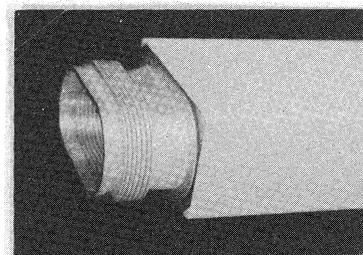
Fig. 5 Ceramic chamber with aluminum bellows for kicker magnet.
