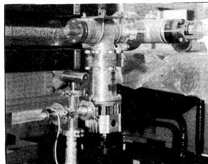
Fig. 13 50 l/s Al-turbomolecular pump for the arc section.
