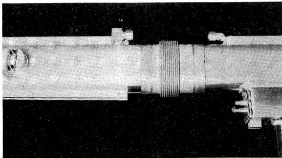
Fig. 1 Assembly of the bending and quadrupole magnets chambers with the bellows. Left side is electrode of beam position monitor.
