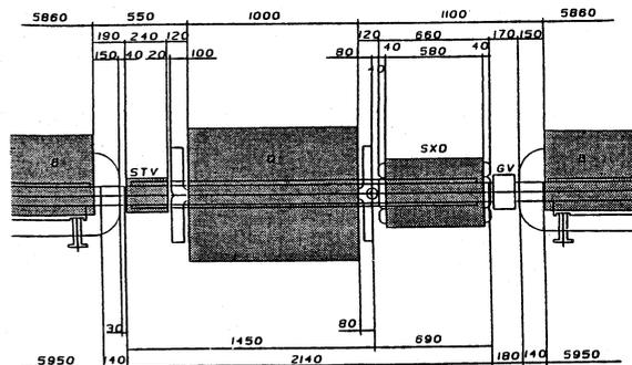
Fig. 10 Layout of the magnets and the vacuum chambers drawn by CAD system.
