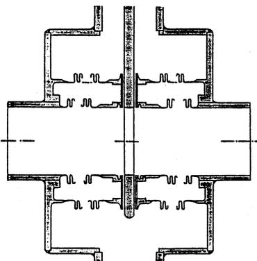
Fig. 6 Dual flat face seal with differential pumping type gate valve.
