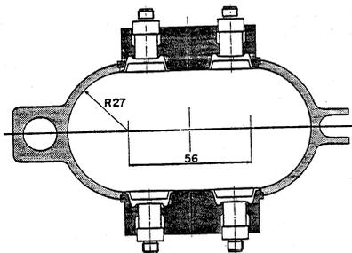
Fig. 8 Beam position monitor mounted on the quadrupole magnet chamber.
