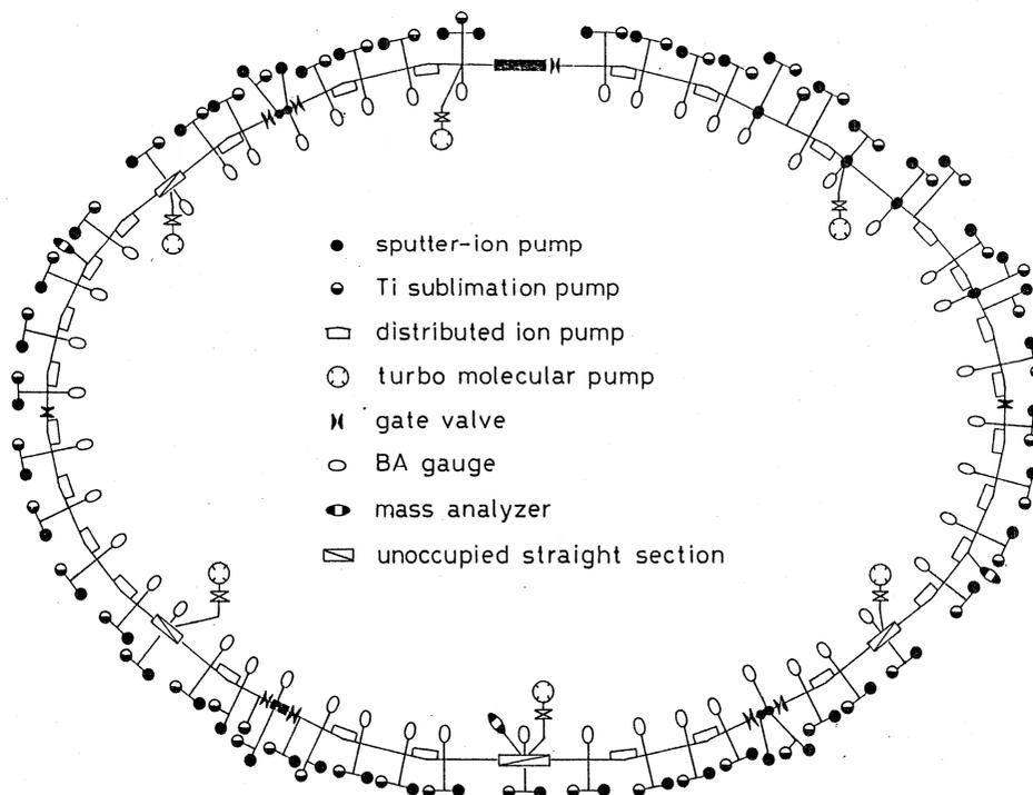
Fig. 1 Schematic illustration of the PF ring vacuum system.
