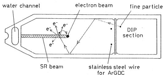
Fig. 5 Process of the trapping of fine particles
