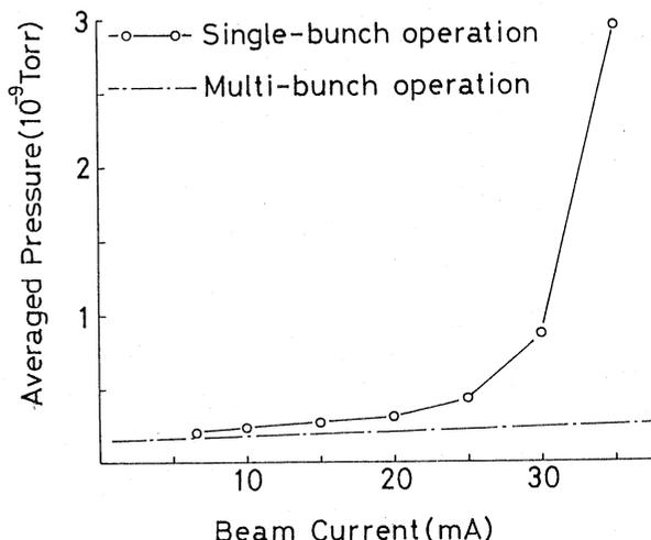
Fig. 6 Beam-current dependences of the pressure in the single-bunch and multi-bunch operations.
