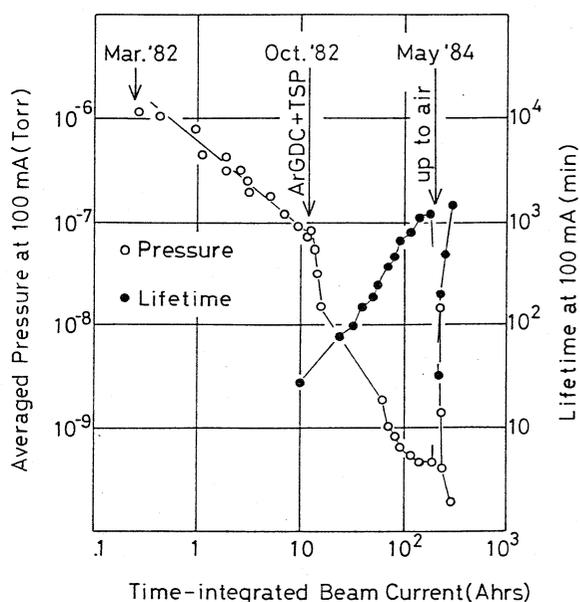
Fig. 2 Decrease of the pressure and improvement of the beam lifetime during the operation of the PF ring.
