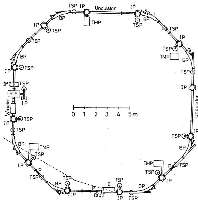
Fig. 1. Plane view of vacuum doughnut of the UVSOR storage ring. IP : sputter ion pump, TSP : titanium sublimation pump, BP : built-in pump, TMP : turbo-molecular pump, RF : RF cavity, P : perturbator chamber, DCCT : DCCT chamber and I : exit of inflector.
