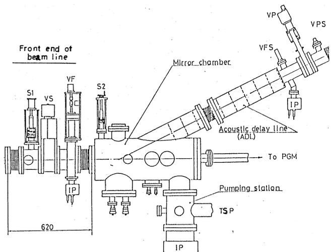
Fig. 4. Side view of BL7B beam line.  $S_1$  and  $S_2$  : water-cooled beam shutter, VS : all metal tightly closing valve, VF : fast closing valve, VP : tightly closing valve with a viton gasket. VFS : sensor for fast closing valve, VPS : sensor for tightly closing valve with a viton gasket, IP : sputter ion pump and TSP : titanium sublimation pump.
