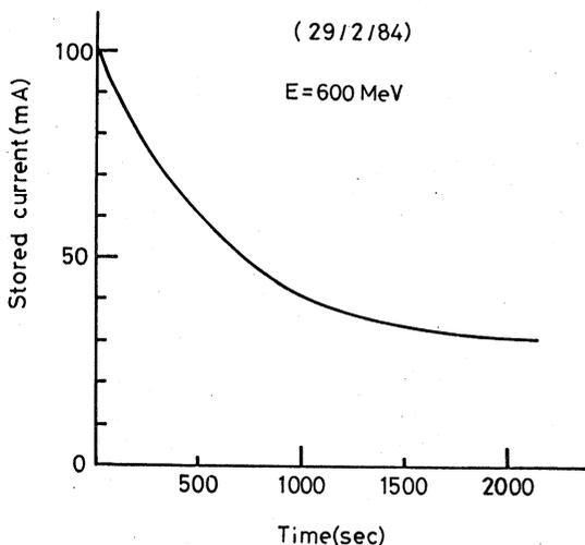
Fig. 3. The decay curve of the stored current of 100 mA.
