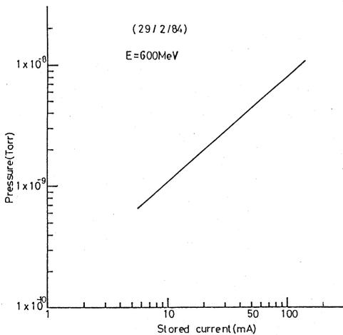
Fig. 2. The dependence of the pressure on the amount of stored current at the injection.
