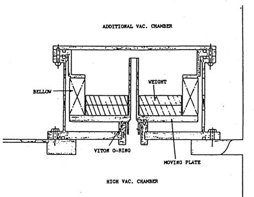
Fig. 3 A fabricated model of the safety valve.
