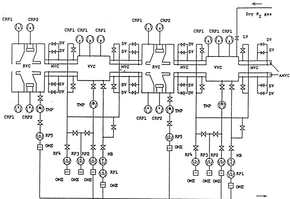
RVC: RF resonator vacuum chamber. MVC: magnet vacuum chamber. VVC: valley vacuum chamber. AMVC: additional magnet vacuum chamber.
