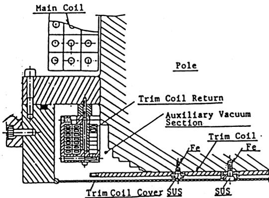
Fig. 2 Cross-sectional view of the pole edge section. Pole surface and trim coils are enclosed in auxiliary vacuum and separated from high vacuum chambers. The main coils are in the atmosphere.
