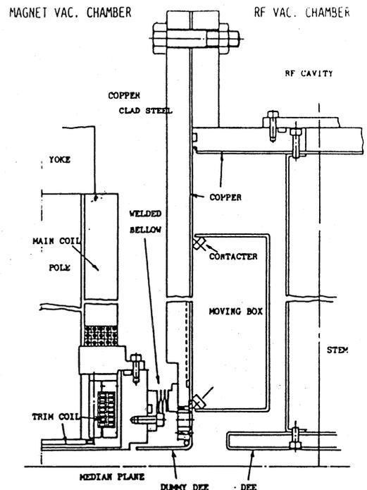
Fig. 5 Sealing method using a welded bellows.
