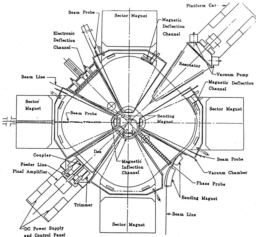
Fig. 1 A plan view of the vacuum chamber of RIKEN SSC.
