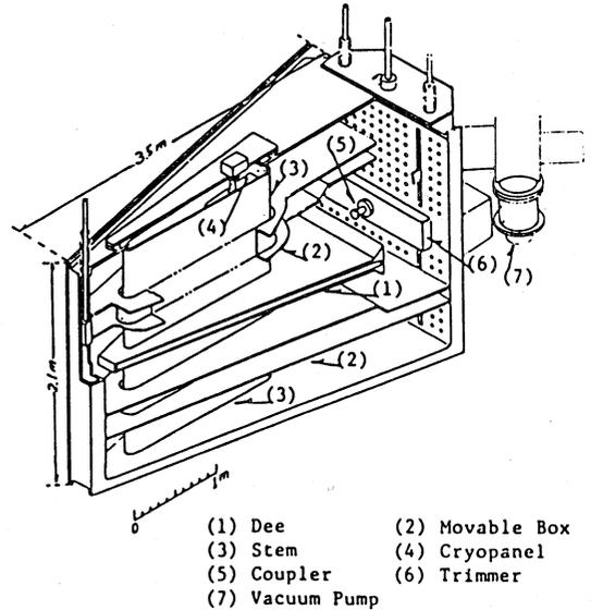
Fig. 4 A bird's-eye view of the RF Resonator for the SSC
