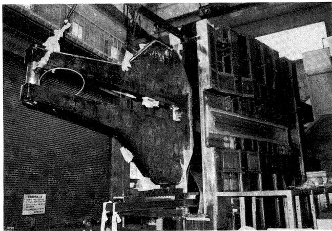
Fig. 4. Rotatable tuner plate being installed into the cavity chamber.
