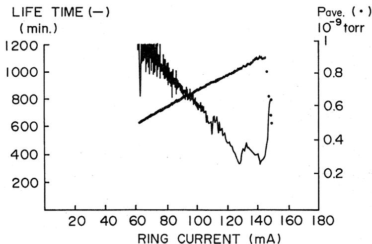
Fig. 4 Beam current dependence of the beam lifetime and the average vacuum pressure.
