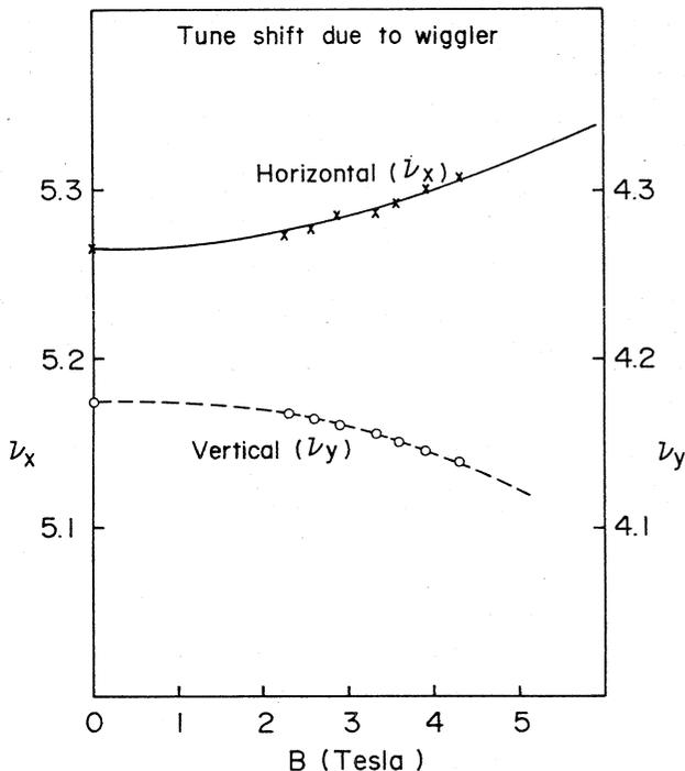
Fig. 3 Variation of the betatron frequency at 2.5 GeV with wiggler excitation,  $\left. \begin{matrix} \circ \\ x \end{matrix} \right\}$  measured, — predicted from parallel pole edge model.
