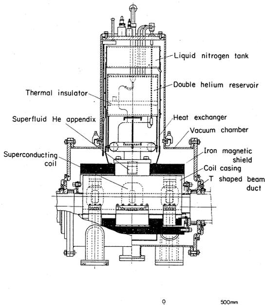
Fig. 1 Cross-sectional view of the superconducting vertical wiggler.
