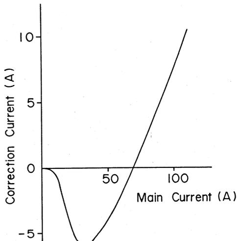
Fig. 2 Correction current as a function of the main magnet current.
