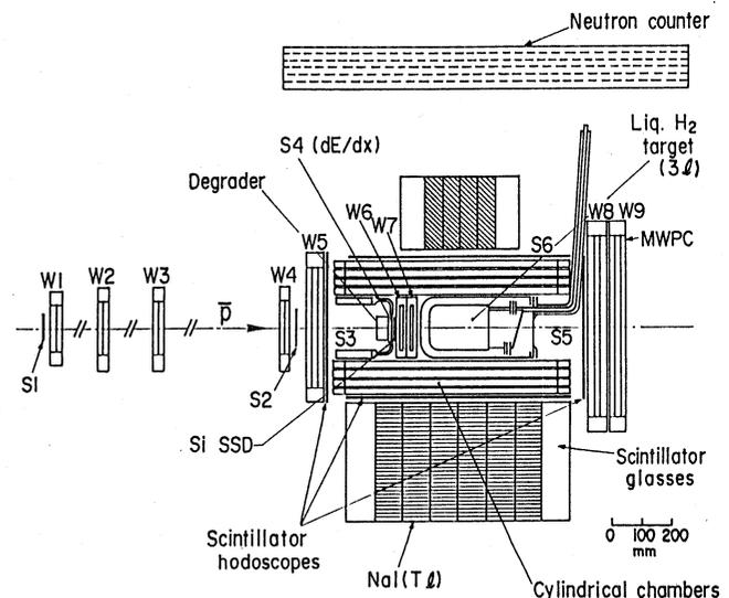
Fig. 2 Setup for E68 experiment.
