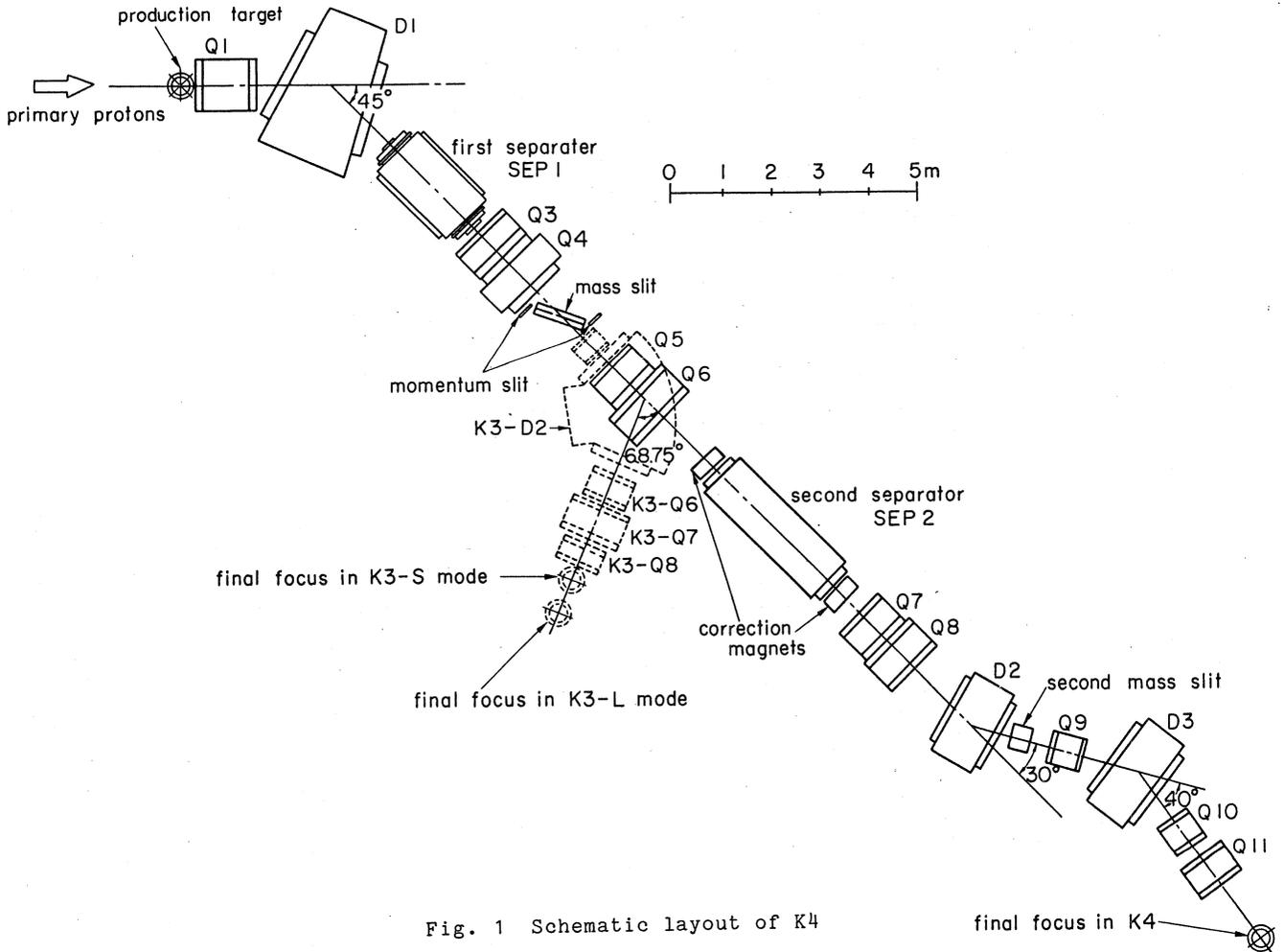
Fig. 1 Schematic layout of K4
