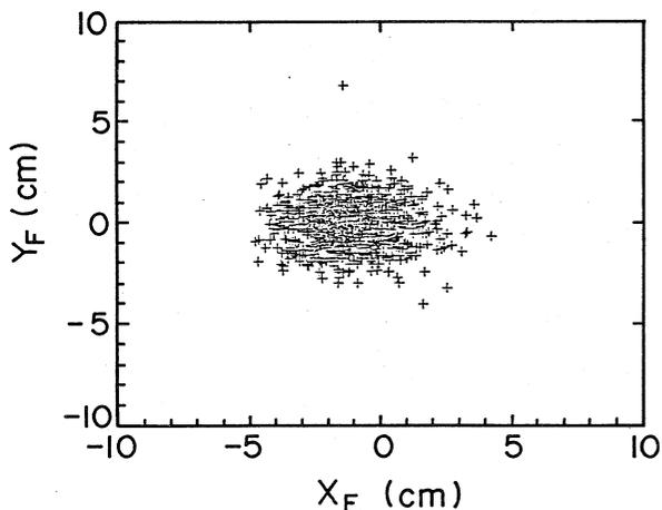
Fig. 3 Beam profile at the center of the hydrogen target.
