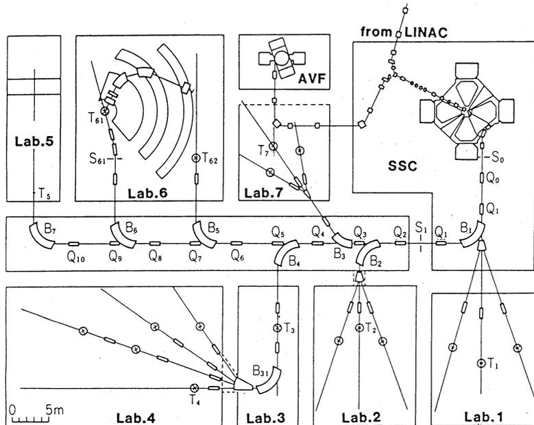
Fig. 3. Plan view of the beam handling system for the RIKEN SSC. S<sub>0</sub> is the object point of the system
