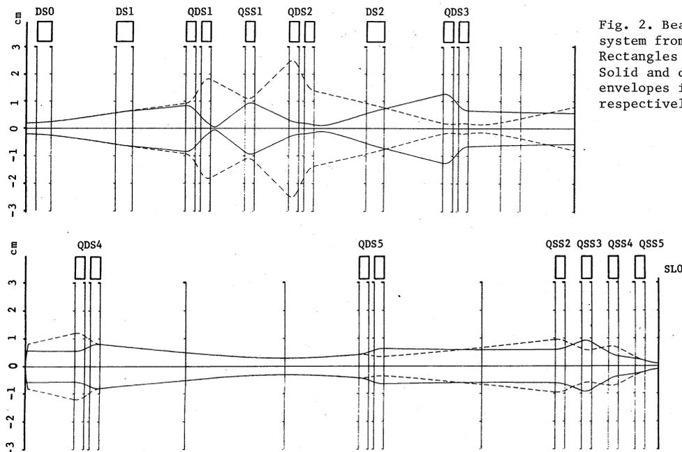
Fig. 2. Beam envelopes through the system from linac to the slit SL0. Rectangles indicate position of magnets. Solid and dashed curves show beam envelopes in the on- and off-midplane, respectively.
