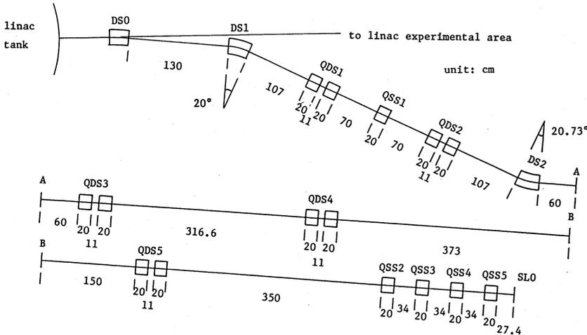
Fig. 1. Plan view of the beam transport system from the linac to the slit SL0.
