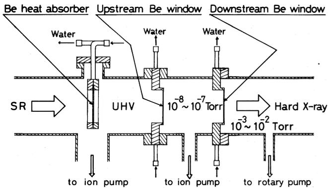
Fig. 4 Schematic of the Be window configuration for the vertical wiggler line.
