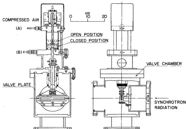
Fig. 2 Cross sectional diagram of the fast closing valve.
