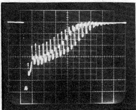
Fig. 5 Output signal of a photomultiplier detecting SR from decaying electrons. The horizontal scale is 2 μs/div.
