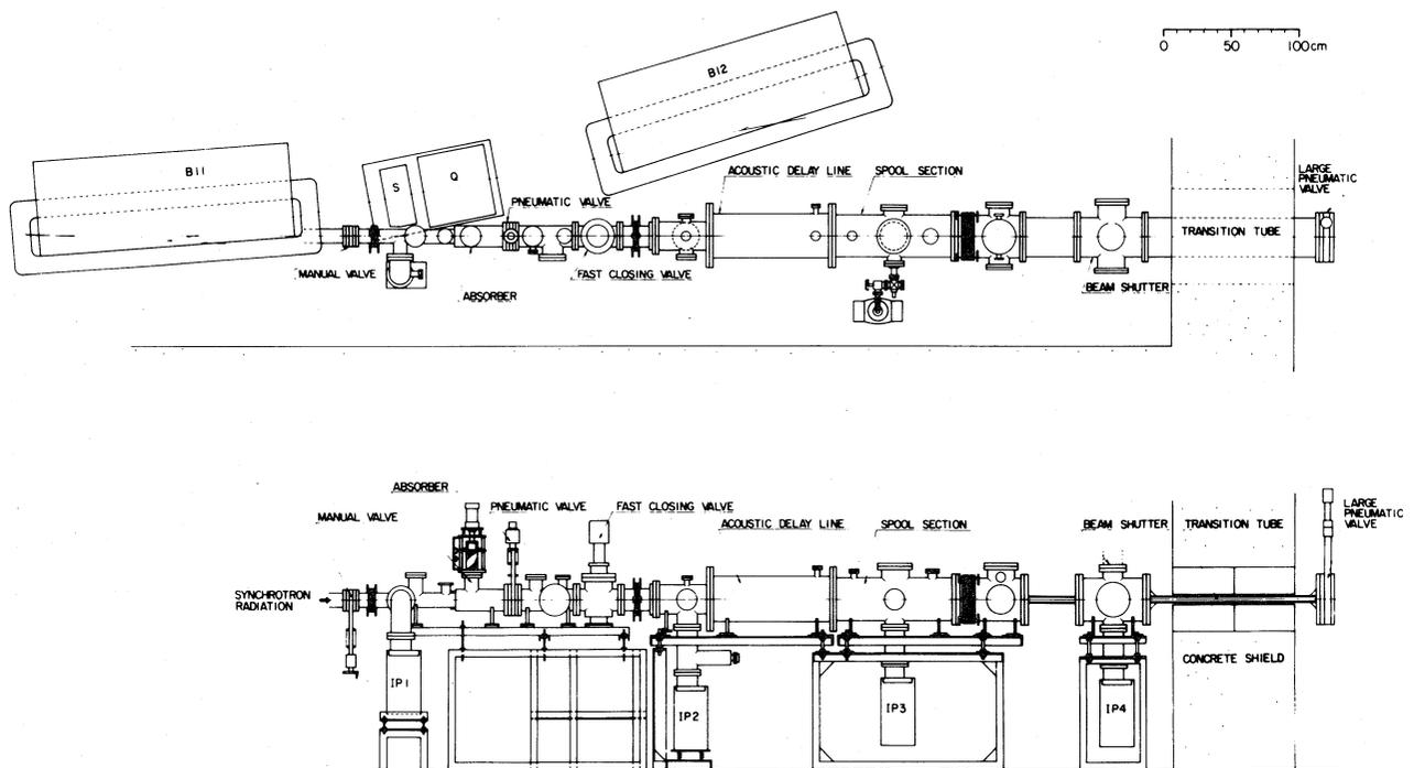
Fig. 1 Layout of the Photon Factory main beam line.
