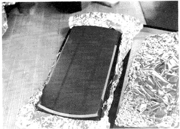
Fig. 6 Pt-coated SiC mirror having been used on the grasshopper line. It has a size of  $40 \times 17 \times 4$  cm<sup>3</sup>.
