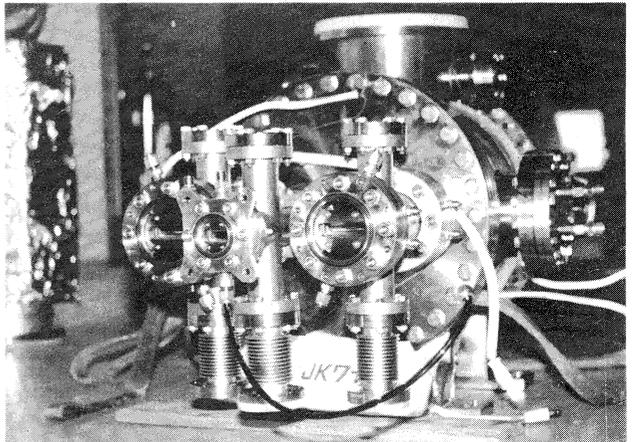
Fig. 7 Be window assemblies having been used on BL-4. The downstream windows are seen.
