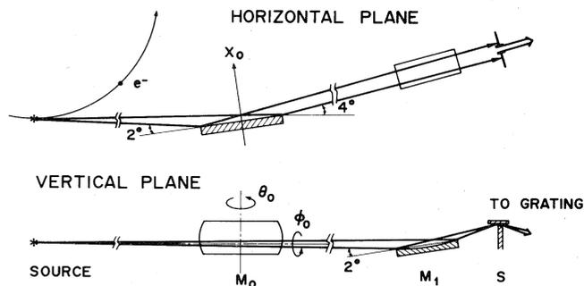
Fig. 3 Optical arrangement of the grasshopper branch line on BL-11.
