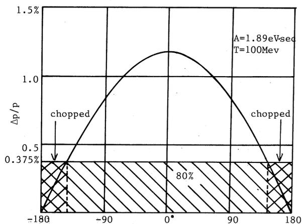
Fig. 1 Stationary bucket and coasting beam
