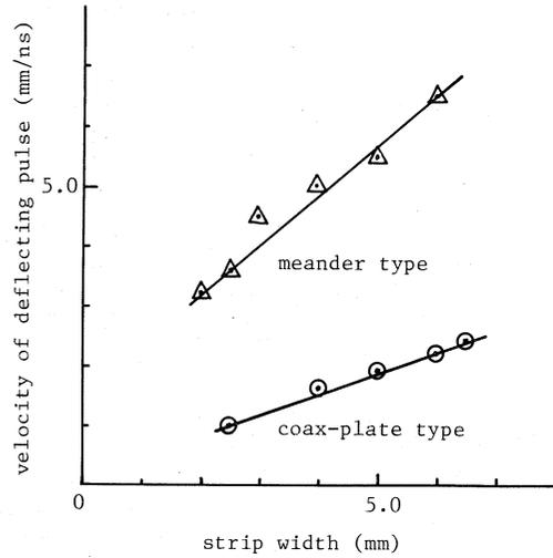
Fig. 6 The longitudinal velocity of deflecting pulse (For coax-plate type, length of coaxial cable is 1.3 times as long as strip conductor.)
