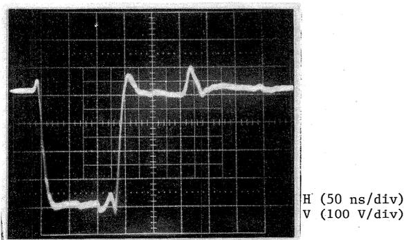
Fig. 9 Photograph of pulse response of a power amplifier
