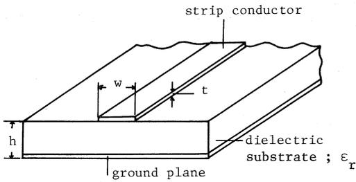
Fig. 4 Schematic diagram of a microstrip transmission line
