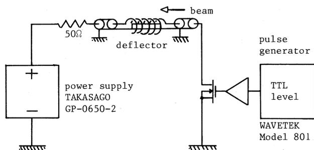
Fig. 8 Schematic diagram of a power amplifier and deflector
