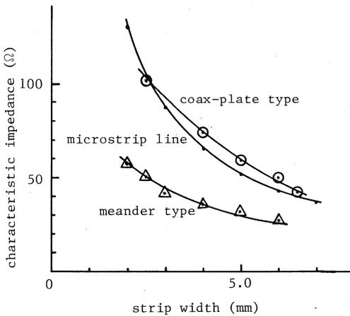
Fig. 5 The characteristic impedances of a microstrip transmission line and each types of deflector (For coax-plate type, the effect of coaxial cable is not taken into account.)
