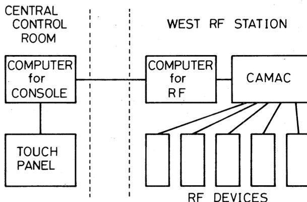
Fig. 2 Block diagram of RF remote control system.
