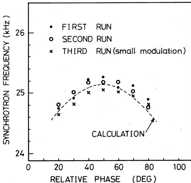
Fig. 3 Measured synchrotron frequency as a function of phase difference between two RF stations.
