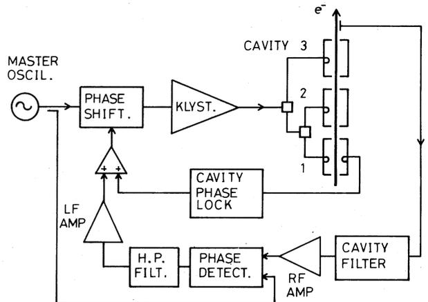
Fig. 4 Block diagram of the feedback system for damping longitudinal dipole oscillations.
