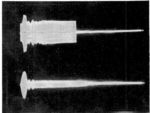
Fig. 10. Typical wave form of the cavity voltage under multipactoring.
