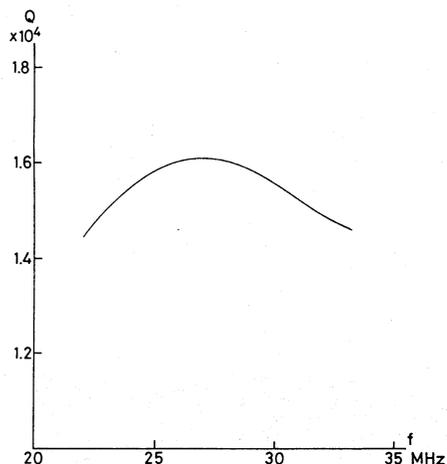
Fig. 6. Q value of H<sub>101</sub> mode resonance vs. frequency.
