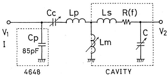
Fig. 8. Equivalent circuit of the output circuit of the RF system.
