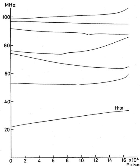
Fig. 5. Resonant frequencies of the cavity vs. position of the tuner plate.
