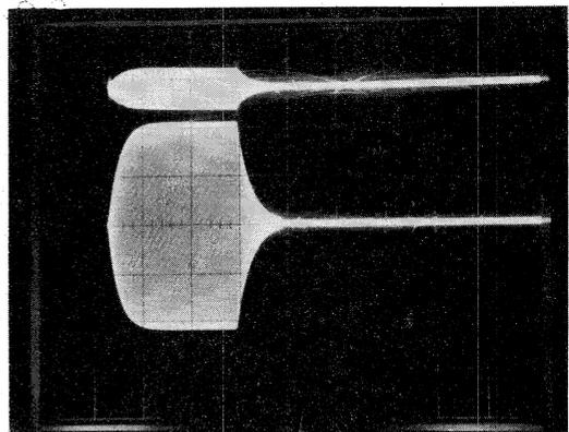
Fig. 11. Typical wave form of the cavity voltage above multipactoring voltage.
