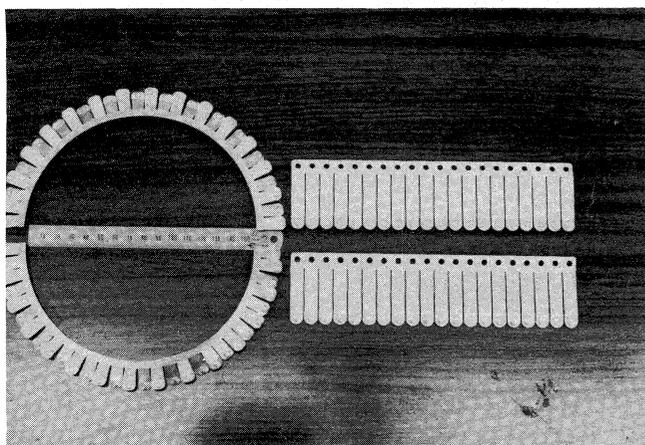
Fig. 4. Photograph of Be-Cu contact springs.
