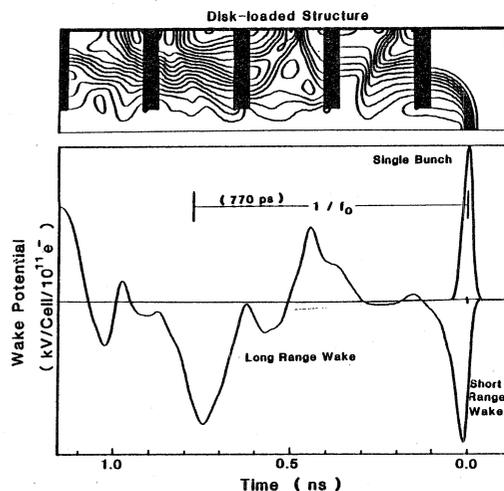
Fig. 7. The wake potential of the single bunch passing through an L-band periodic structure. The bunch length is 4 mm.
