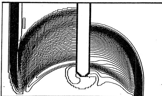
Fig. 6. Wakefields generated by a single bunch passing through a disk-loaded structure. The bunch length is 2 mm long, while the thickness of the disk is 13 mm.
