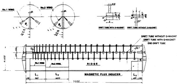
Fig. 2 The Structure of the first lineac cavity.
