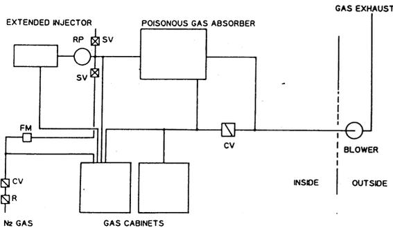
Figure 9. Gas cabinets, a poisonous gas absorber and a gas blower. RP; Rotary pump, SV; Stop valve, FM; Flow meter, CV; Check valve, and R; Regulator.
