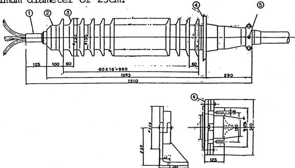
Figure 5. Outlines of the high voltage cable head in air. (1) Brass terminal tube, (2) Rubber cap, (3) Rubber shell, (4) Aluminum cover, (5) Screw hole for an earthing terminal, and (6) Supporting bracket.
