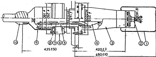
Figure 4. A cross-section of the high voltage cable terminal in gas. (1) Shield ring, (2) Metal conductor, (3) Insulating epoxy resin tube, (4) Rubber insulator, (5) FRP pipe, (6) Insulating ring, (7) Compressing spring of the rubber insulator, (8) Flange, (9) Metal cap for protecting the cable, and (10) Water proofed tape layer.
