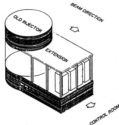
The extension has a lower column only as it is shown in fig.1. On the other hand, the old injector has both upper and lower columns.
