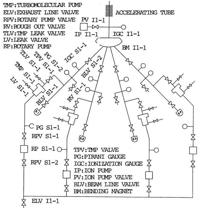
Figure 7. New vacuum system of the extended injector.
