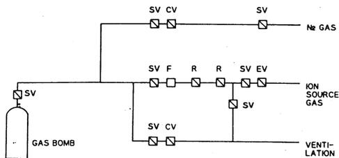
Figure 10. A gas panel for handling harmful gases. SV; Stop valve, CV; Check valve, F; Filter, R; Regulator, and EV; Emergency stop valve.
