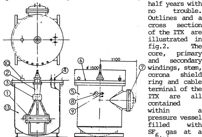
Figure 2. Outlines and a cross-section of the SF<sub>6</sub> gas insulated high voltage isolation transformer. (1) Isolation transformer, (2) Insulating epoxy resin tube, (3) Shield ring, (4) Primary leads, (5) Pressure vessel, (6) Top flange of the vessel, (7) Manway, (8) Bourdon tube pressure gauge, (9) Gas manifold, and (10) Gas relief valve and rupture disc.
