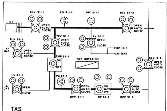
Figure 8. A diagrammatic display of the S1 mini-beam line.
