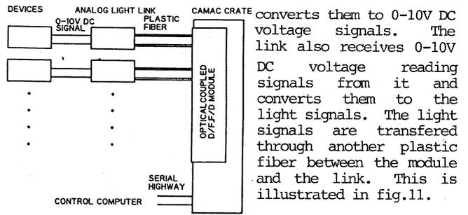
Figure 11. An illustration of an optical coupled D/F.F/D module, plastic fibers and analog light links used for controlling the devices in the high voltage racks.
