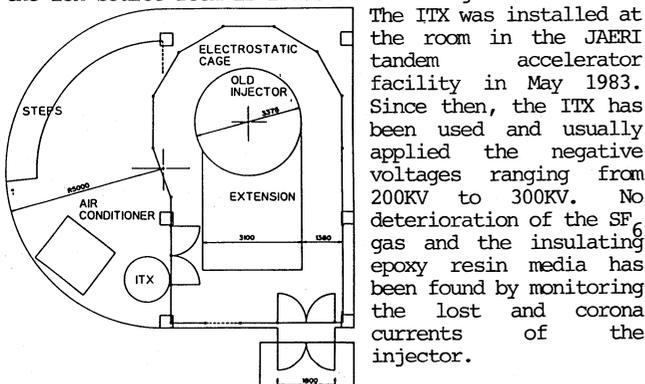
Figure 6. Arrangement of the ITX and the extended injector in the ion source room of the JAERI tandem accelerator facility.
