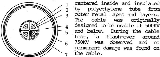
Figure 3. A cross-section of the high voltage cable. (1) Four conductors of copper wire having a 90° sector and 25mm<sup>2</sup> cross-section, (2) Polyethylene insulator, (3) Semiconductive tape and layer, (4) Polyethylene insulator, (5) Semiconductive tape and layer, (6) Copper tape and compressing tape, and (7) Polyvinyl chloride jacket.
