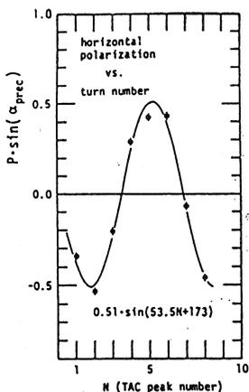
Fig. 5 Horizontal polarization as a function of the peak number in the TAC spectrum for 65 MeV protons.
