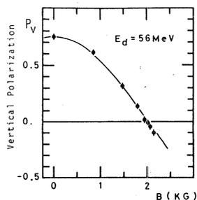
Fig. 3. Vertical polarization of deuteron as a function of the magnetic field of the Wien filter.
