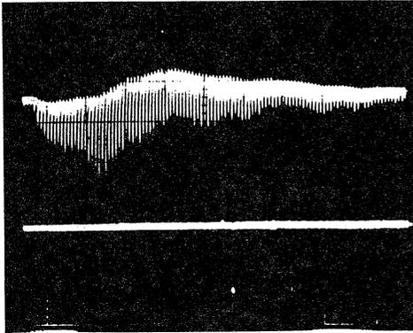
Fig. 4. Distribution of the turn numbers at a duty cycle of 1/115 observed for 56 MeV deuterons. The upper curve indicates signals from the plastic scintillator in the beam path, and the lower curve shows the trigger signal from the frequency divider. The horizontal scale is 1  $\mu$ s/division.
