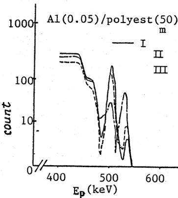
Fig.3 RBS spectra for protons incident on Al/Polyester films. I, II, III correspond to the parts shown in Fig.2.
