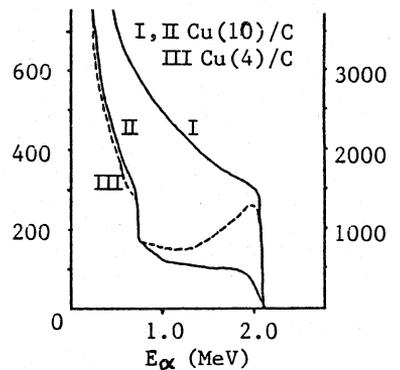
Fig.6 RBS spectra for He-ions incident on Cu/C, I: before, II: after irradiation, and Cu/C 4 m/2mm III after irradiation.
