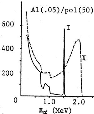
Fig.5 RBS spectra for He-ions incident on Al/PE film; I: before and II: after irradiation.
