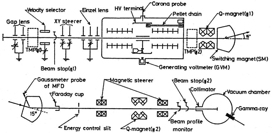
Fig.1 A schematic diagram of the accelerator and the 7m-beam line.
