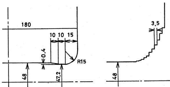
Fig.1 Shape of pole tip of the bending magnet.
