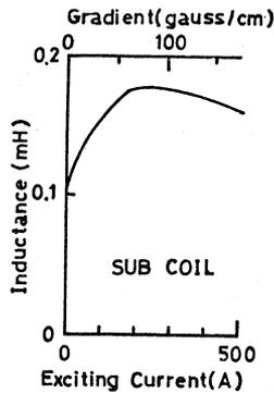
Fig.6 Dependence of the inductance upon the exciting current.
