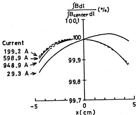
Fig.2 Dependence of the integrated field along the orbit upon radial displacement (x).
