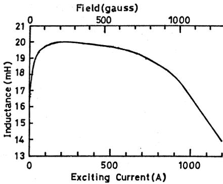
Fig.3 Dependence of the inductance upon the exciting current.
