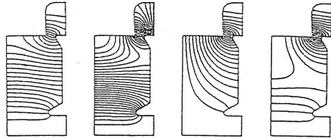
Fig. 2 Electric Field of Type B Cavity. 0-mode,  $\pi$ -accelerating Mode,  $\pi$ -Coupling Mode and  $2\pi$ -mode (L-R).
