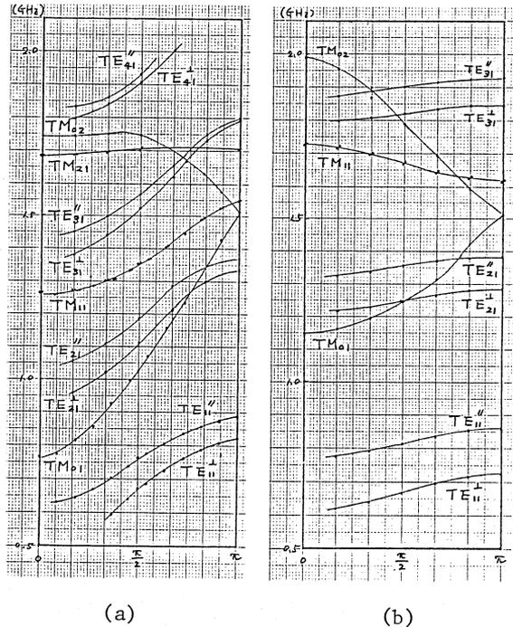
Fig. 3 Dispersion Curves of (a) Type A and (b) Type B Cavity.
