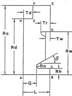
Fig. 1 Geometrical Notation of a Half-cell DAW Cavity.
