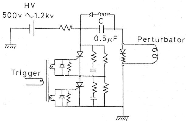
Fig. 3 Diagram of the circuit for the pulser of the perturbator.
