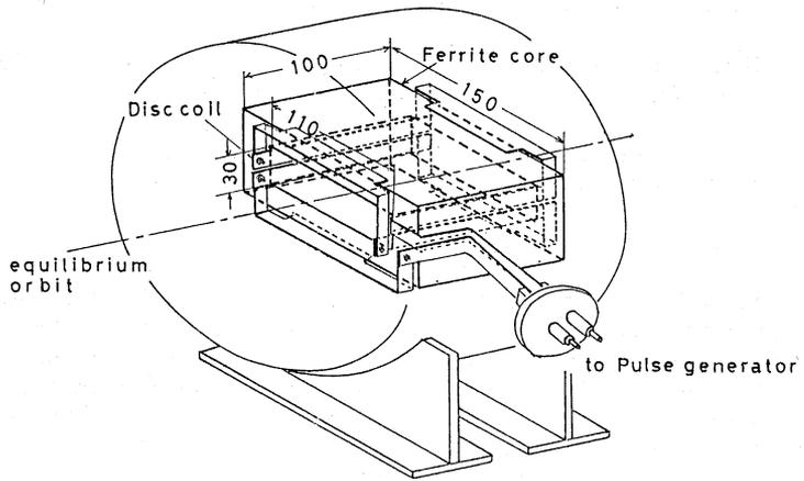
Fig. 2 Perspective view of the perturbator.
