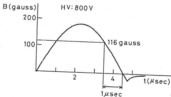
Fig. 4 Magnetic field waveform at the center of the perturbator.
