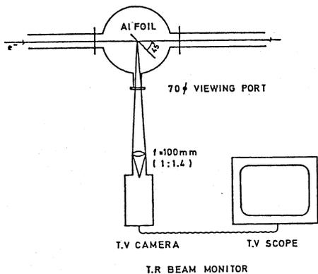
Fig.1 Block diagram of the T.R beam position monitor.
