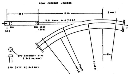
Fig.2 Layout of the SPD stored current monitor.
