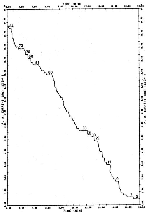
Fig.3 Decay step of SR intensity observed by the PM beam current monitor.
