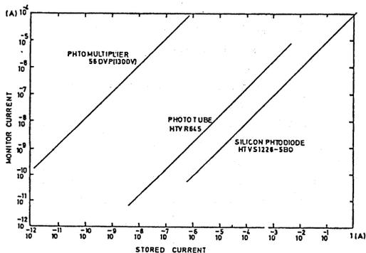
Fig.4 The monitor responses versus stored current.
