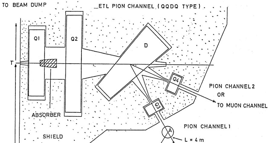
Fig. 3 Layout of the ETL pion channel
