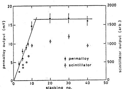
Fig.2 Intensity of stored current is measured with permalloy monitor and scintillation monitor. Intensity increases linearly up to the stacking number of 15.
