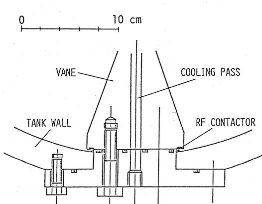
Fig. 2. Contact of vane and tank.
