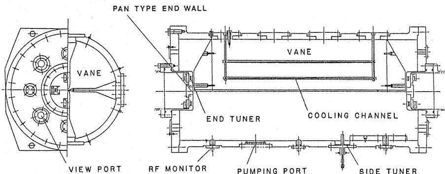
Fig. 1. View of the RFQ cavity of LITL.
