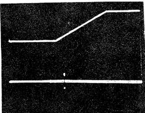
(a) Upper; Sweep signal of RF frequency for stacking, Lower; the pulsed RF.
