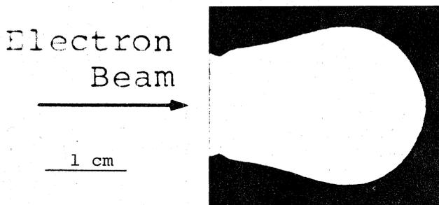
Fig. 3. An experimental isodose curve in an aluminium cylinder for a collimated 15-MeV electron beam. The isodose curve is recorded in a mica sheet(right).
