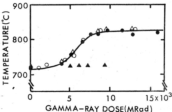
Fig. 2. Resistance to thermal decomposition of muscovite mica as a function of absorbed gamma-ray dose. ● gamma-ray irradiation, ○ electron irradiation, ▲ gamma-ray irradiation (160°C-170°C), △ annealed after one year of storage from the end of the gamma-ray irradiation.
