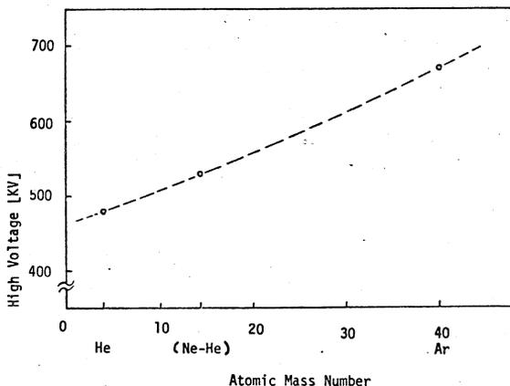
Fig. 3, Mass number dependence of the breakdown voltage at the pressure of  $1 \times 10^{-4}$ .
