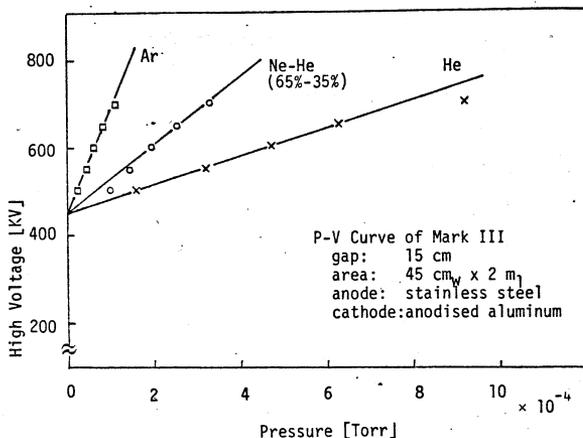
Fig. 2, Pressure dependences of the breakdown voltages for the gases of Ar, Ne-He and He at the separator Mk-III.
