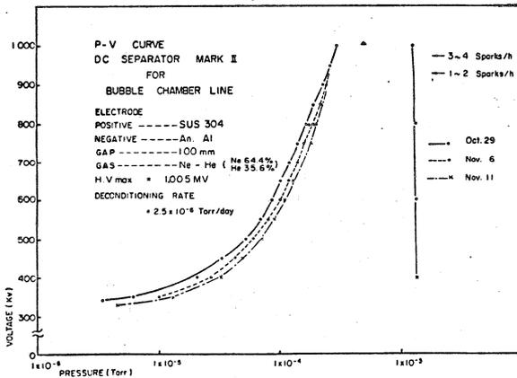
Fig. 1, Pressure dependence of the breakdown voltage at the electrostatic separator (Mark II-2).
