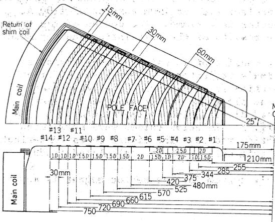
Fig. 2. Configuration of the trim coils for the model magnet
