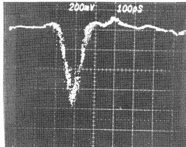
Phot.5 Pulse shape of the picosecond single pulse with small satellites measured by using the micro strip line monitor.
