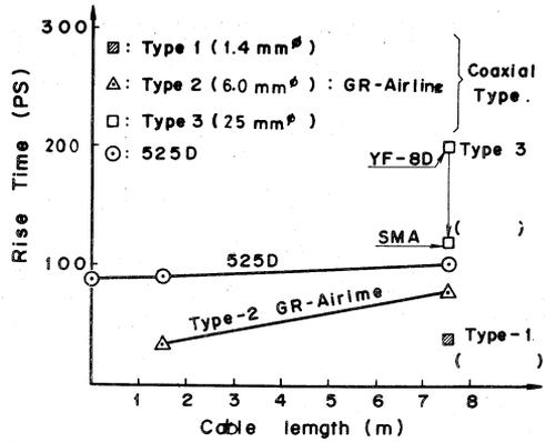
Fig-1 Dependence of response on both detector head and connecting cable length.
