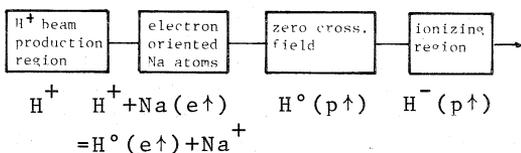
Fig.1 Block diagram of pol. H<sup>-</sup> ion source
