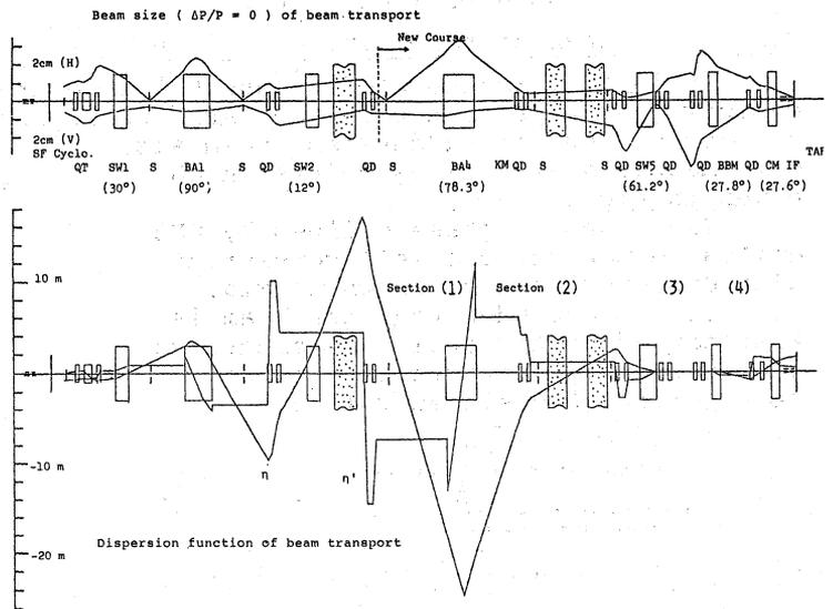
Fig.1 Beam envelopes and dispersion functions
