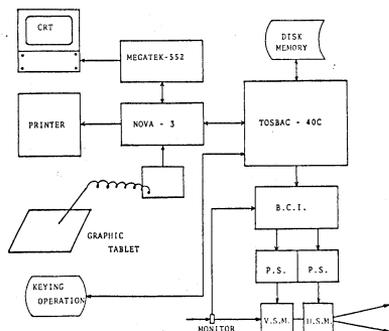
Fig.2. Spot scanning data input and controll system.
