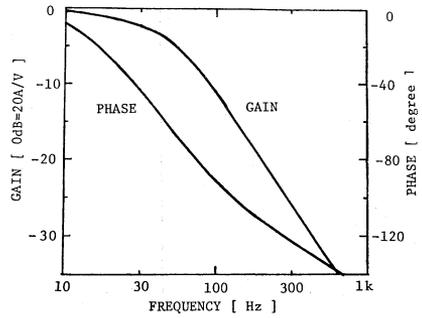
Fig.2 Frequency response of bump power supply.
