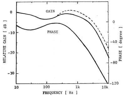
Fig.4 Estimated loop gain of servo-spill system.
