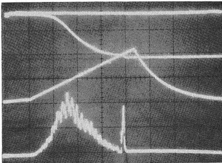
Fig.5 A photo of the beam spill without servo. The traces are circulating beam current, current of bump magnet, and output of spill monitor. (Horizontal=100msec)
