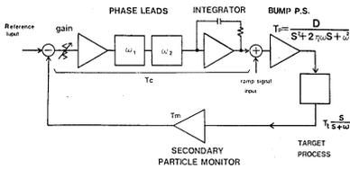
Fig.3 Block diagram of servo-spill system.
