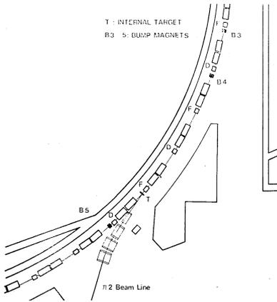
Fig.1 Layout of bumps and internal target in the main ring.
