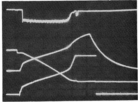
Fig.6 A photo of the beam spill with servo. The traces are output of spill monitor, circulating beam current, current of bump magnet, and output of connecting circuit. (Horizontal=100 msec)
