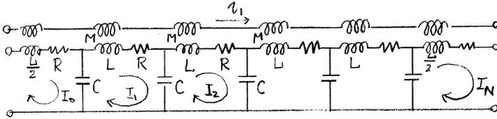
Fig.2 Equivalent circuit of the magnet with a primary current
