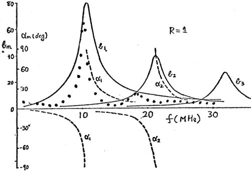
Fig.3 Induced voltage  $b$  and phase lag  $\alpha$ . The dots<sup>m</sup> in the figure is the measured.
