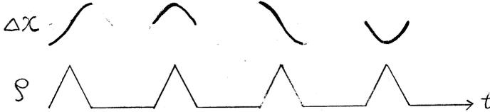
Fig.4 A simplified model of the bunched beam.
