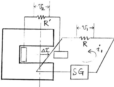
Fig.1 Setup of the measurement of induced voltage by a primary current.
