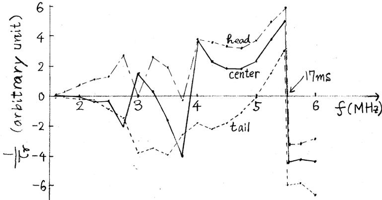
Fig.5 Build up of damping time during acceleration.
