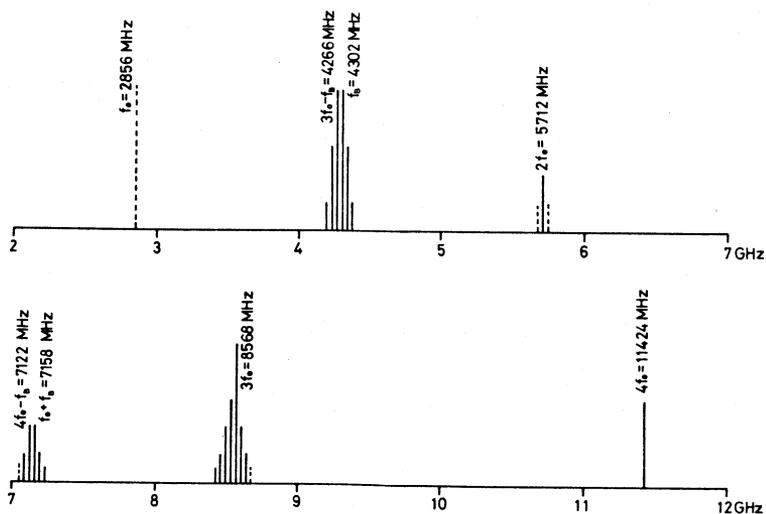
Fig.5 Frequency spectrum of the beam with BBU.
