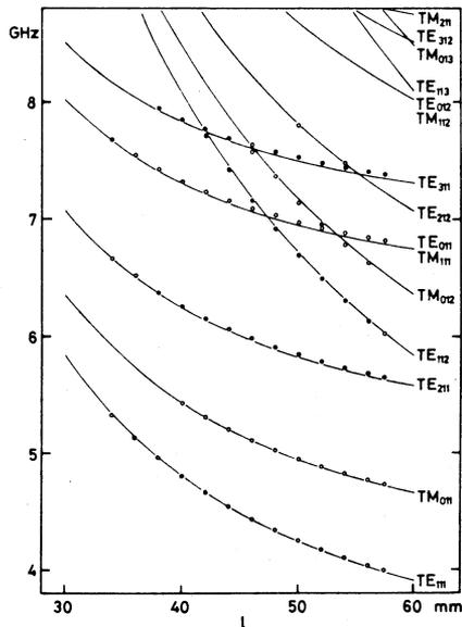
Fig.2 Various mode resonant frequencies vs. axial length of the cavity.
