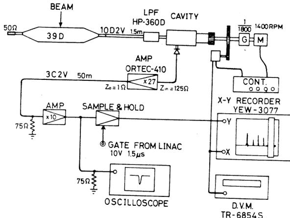
Fig.1 Block diagram for measurement of frequency components.
