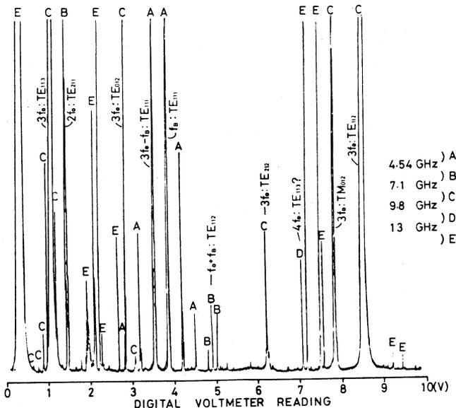
Fig.3 Frequency components involved in the beam modulated by BBU.
